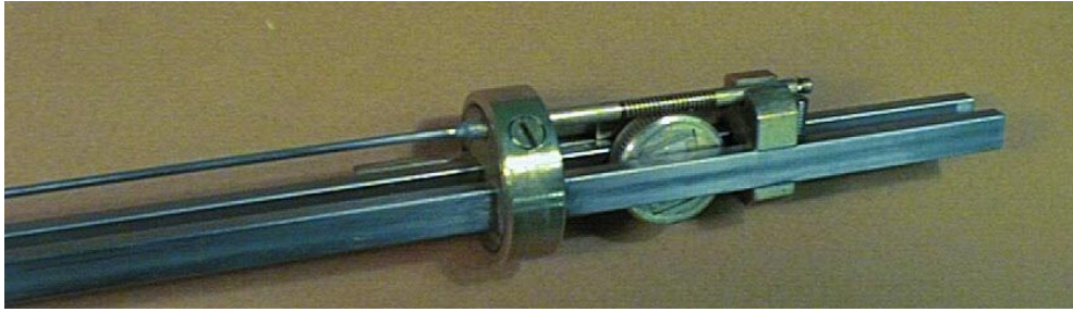
Figure 7. Detail of the cryogenic insert designed to rotate the rectangular resonant cavity and sample in a quasistatic magnetic field. The rectangular cavity is visible within the brass cogwheel; it pivots about the Rexolite cylinders which also couple the cavity to the waveguides (see figure 6). The worm drive which turns the cogwheel is at the top of the picture. The wedge that clamps the cavity tightly between the waveguides is just visible behind the rearmost waveguide.
